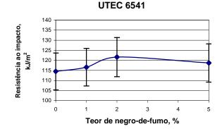
Figure 11: Influence of the CB concentration in the resistance of the impact of
